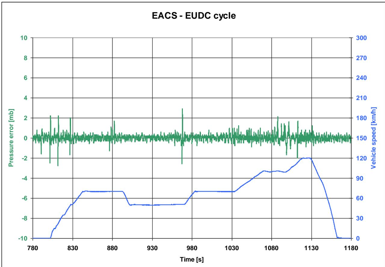
The following diagram shows the pressure inside the volume in the case of extreme engine running conditions.
