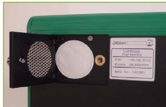
**For fine dust analysis in highest precision** ranging from 0.25 to 32  $\mu\text{m}$  in 31 size channels, this top of the line device is unique and has no equal! The areas of use range from fine dust monitoring in industrial and manufacturing facilities to workplace measurements. With the advanced data communication interfaces, the **Mini-LAS 11-E** offers its users utmost flexibility and mobility.
