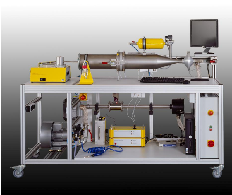
Filter Tests with the Automated Test Rig AFC 131
