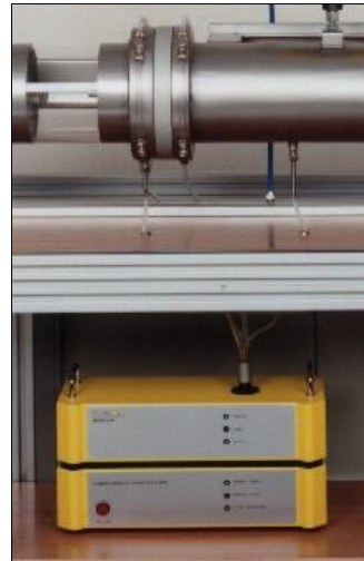
Efficiency Measurement with the LAP 321 Optical Particle Counter placed under the Test Channel below the Switching Valve
