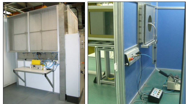
Mixing chamber with air intake filter and aerosol generation (droplet aerosols and dust); right: interior view
