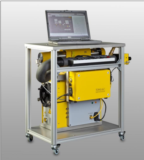
The Blow-By Test Rig BBT 143 for measuring the oil concentration of blow-by gases: Gravimetric Measuring System GMS 141, Process Aerosol Photometer PAP 610 and PAP 612
