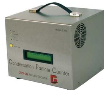
The CPC from Grimm can be used as a stand-alone instrument in combination with a dilution system, or as part of an integrated measurement system (see description of the RS-PMP instrument below). In the latter case, a specially developed CPC instrument is provided by Grimm.
