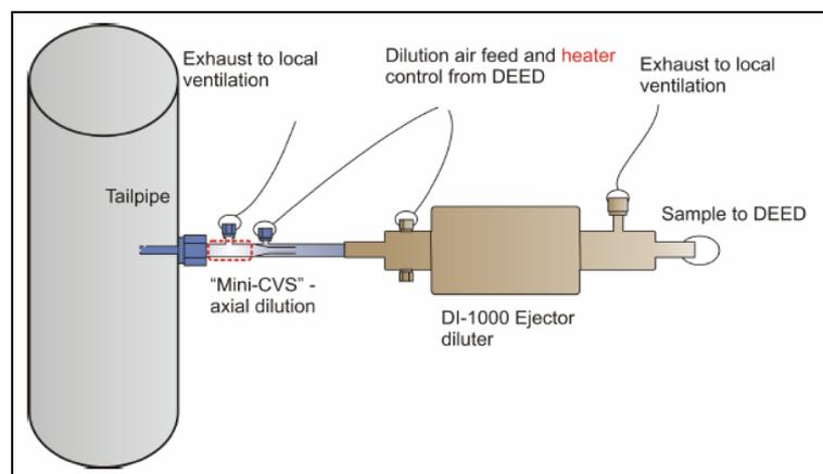
The alternative dilution systems described above can provide similar result as the PMP dilution regarding volatile particle removal of but with far less complexity and thus, they are much more cost-effective than fully PMP-compliant dilution systems. Contact us for more information about how to customize a solution for your particular measurement application.
