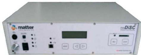
current amplifiers measure the current from the mentioned stages. A calculation of particle number and size (20 to 200 nm interval) is made. Among the features of the meDisc instrument are that it is portable, robust and easy to use.
