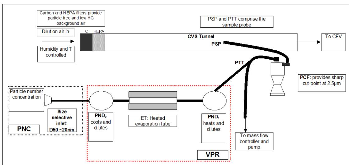
The measurement system comprises, among other things, a volatile particle remover (VPR) as one of the most important sub-systems. The VPR has a first hot stage of dilution (PND1) and a second cold stage (PND2) with an evaporation tube (ET) in
