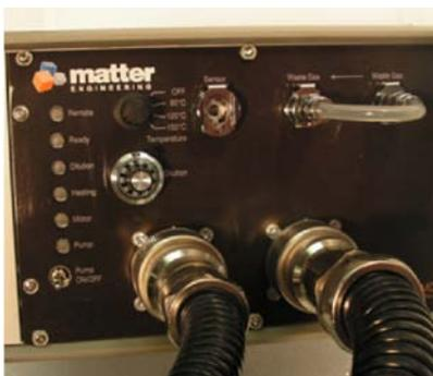
The rotating disk diluter provided by Matter Engineering of Switzerland was the first commercial measurement system developed for PMP measurements. It was used as the “golden” measurement system in the PMP programme for light-duty vehicles. Thus, it is probably one of the best characterised measurement systems, which has manifested itself in numerous publications.
