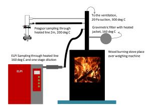
trap voltage setting. A higher trap voltage was used during this experiment to have a higher cut point and to provide the best accuracy for PM measurement. The soot emission from small scale combustion device is expected to vary between different systems hence the M-Sensor should be calibrated for PM against gravimetric PM measurement specific to the system under measurement.
