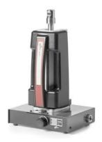
used for chemical analysis of the collected sample. The DLPI+ operates at a sample flow rate of 10 lpm. DLPI+ comes with the data processing spreadsheet for analysing the results.
