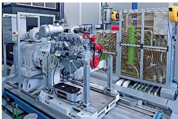
The test cell is equipped with instruments for gas analysis of regulated emission components (Horiba MEXA 7200D), unregulated components (V&F mass spectrometer), particulate matter gravimetrically and real-time (PSS-20 with Pegasor PPS-M sensor), particle number (MEXA 2000 SPCS) and an
