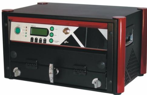
distribution (mass median size and geometric standard deviation). With a detection limit below  $1 \mu\text{g}/\text{m}^3$ , DMM provides better resolution than competing instruments in this field. Furthermore, DMM measures not only soot but all particles. Preferably, volatile particles can be removed in the dilution process to mimic the PMP sampling conditions for solid particle measurement, as described above.
