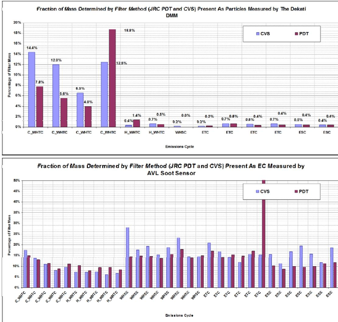
**Figure 1.** Fraction of mass determined by filter method presented as solid particles by DMM (upper graph) and elemental carbon by DMM (lower graph)
